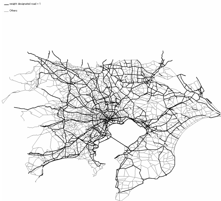
Figure 5 Heavy trucks permitted links in Tokyo
