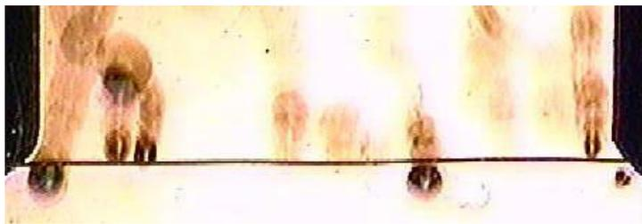
Fig. 4 Boiling behavior on bare surface at heat flux of 0.2 MW/m<sup>2</sup> under earth gravity
