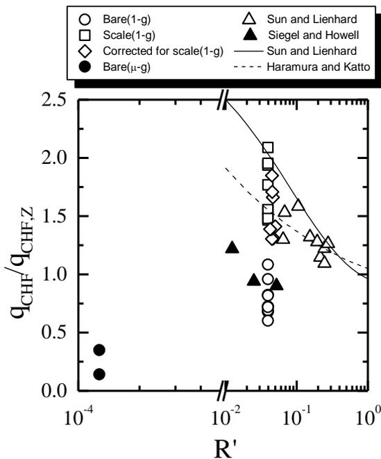
**Fig. 14 Effect on heated surface size on bare and scale surface under earth gravity and microgravity**
