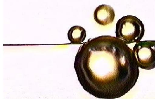
**Fig. 9 Boiling behavior on bare surface at heat flux of 0.12 MW/m<sup>2</sup> under micro gravity**
