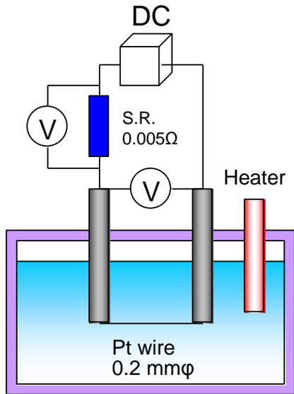
**Fig. 1 Schematic of experimental apparatus**
