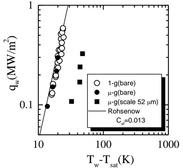
**Fig. 13 Boiling curves on bare and scale surface under micro gravity**
