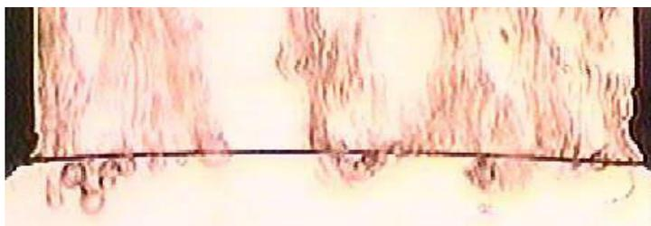
Fig. 5 Boiling behavior on scale surface at heat flux of 0.2 MW/m<sup>2</sup> under earth gravity
