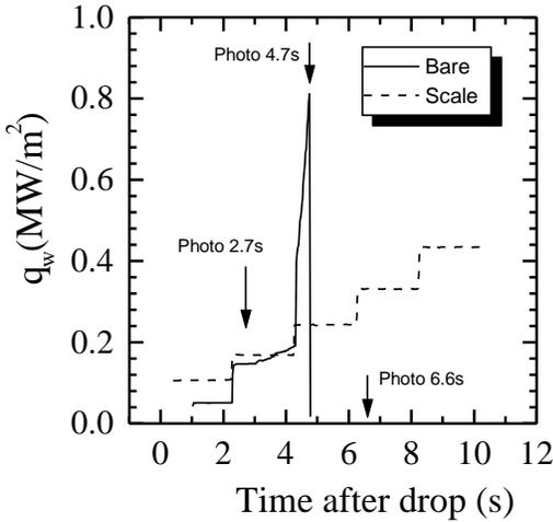
**Fig. 11 Low heat flux burnout of bare wire under micro gravity**
