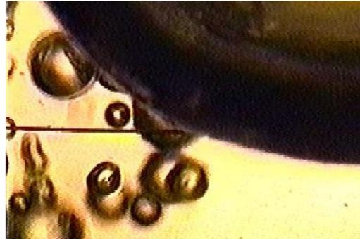
**Fig. 10 Boiling behavior on scale surface at heat flux of 0.12 MW/m<sup>2</sup> under micro gravity**
