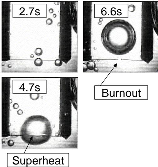
**Fig. 12 Photographs for low heat flux burnout of bare wire under micro gravity**
