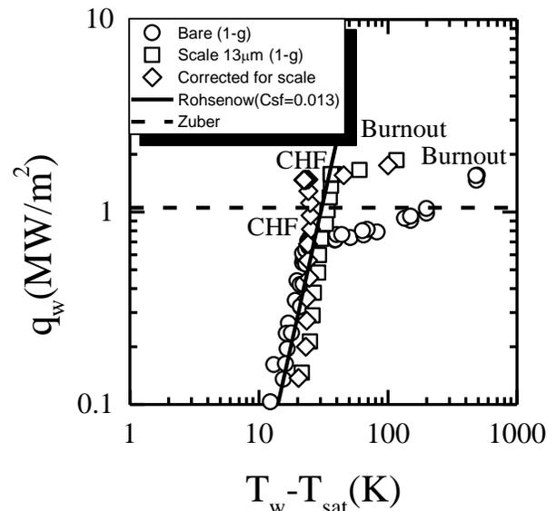
Fig. 8 Boiling curve on for bare surface and scale surface under earth gravity
