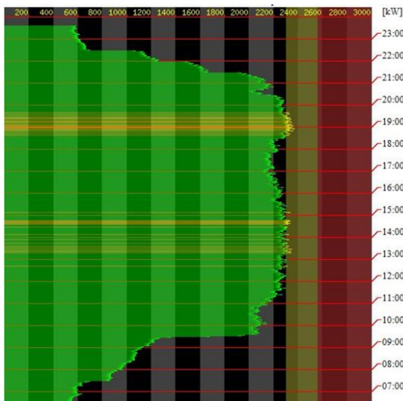
Fig.7 Display of electricity demand on web
