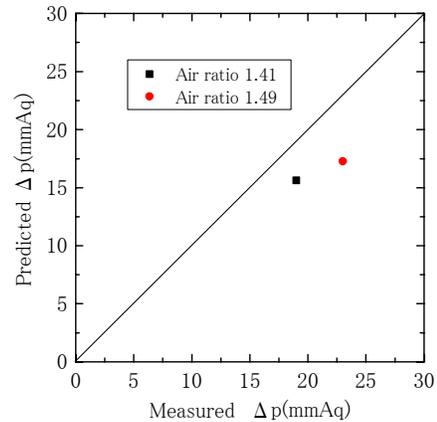
**Fig. 5 Pressure difference between inlet and outlet of heat exchanger**
