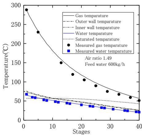
**Fig. 4 Temperature distribution in compact heat exchanger**
