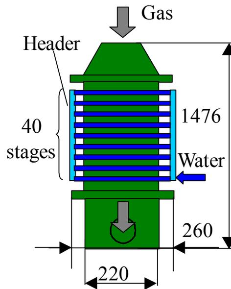
Fig. 2 Schematic of experimental apparatus for compact heat exchanger
