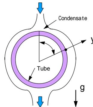
Fig. 7 Heat conductance of condensate film
