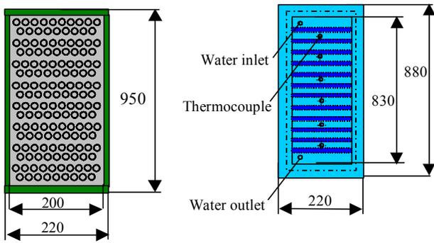
**Fig. 3 Cross-section of compact heat exchanger using Small Tubes**
