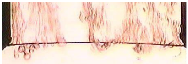
Fig. 5 Boiling behavior on scale surface at heat flux of 0.2 MW/m 2 under earth gravity
