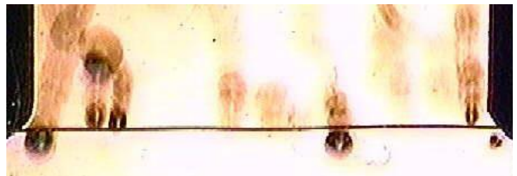
Fig. 4 Boiling behavior on bare surface at heat flux of 0.2 MW/m 2 under earth gravity
