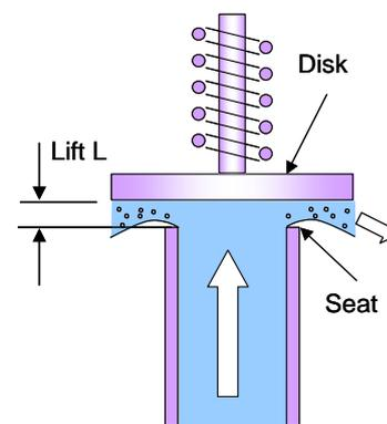
Fig.1 Disk-type flow contraction
