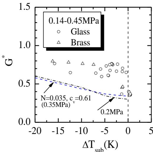
Fig.14 Mass flux of subcooled liquid
