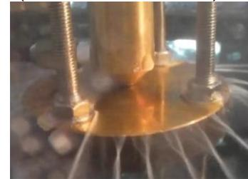
Fig.8 Discharging behavior in taper seat ( $L=0.3\text{mm}$ ,  $\Delta P=0.3\text{MPa}$ )
