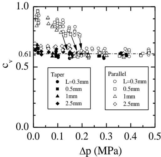
Fig.5 Relation between discharging coefficient and pressure difference
