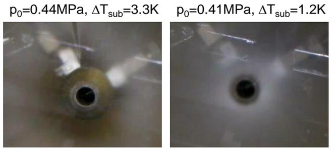
Fig.15 Flashing behavior of subcooled liquid
