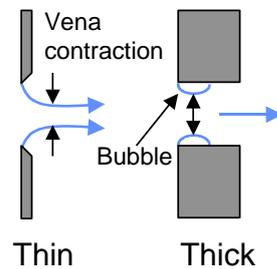
Fig.4 Flow through orifice
