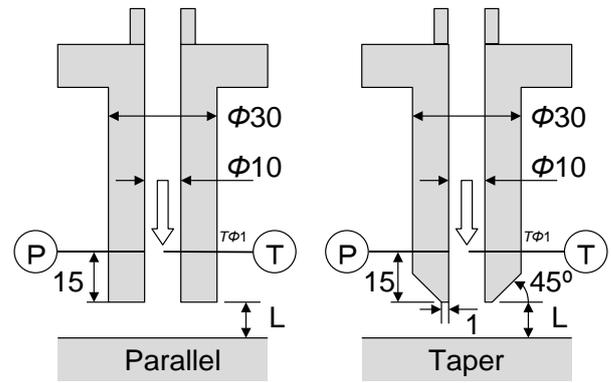
Fig.3 Valve seat configuration
