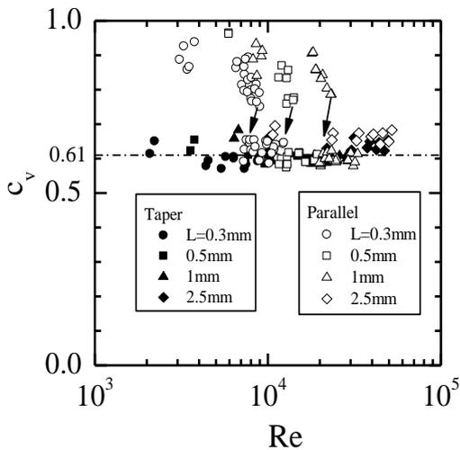
Fig.6 Relation between discharging coefficient and  $Re$
