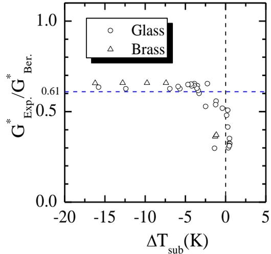
Fig.16 Ratio of experimental mass flux to Bernoulli prediction of subcooled liquid
