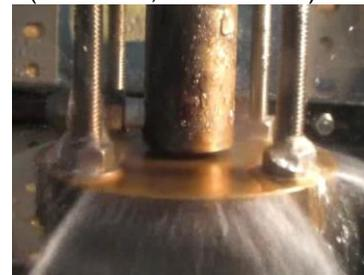
Fig.9 Discharging behavior at larger lift in parallel seat ( $L=2.5\text{mm}$ ,  $\Delta P=0.1\text{MPa}$ )
