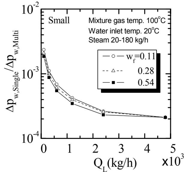
Fig. 10 Ratio of pressure loss in water side at different water flow rate in “Small” HX
