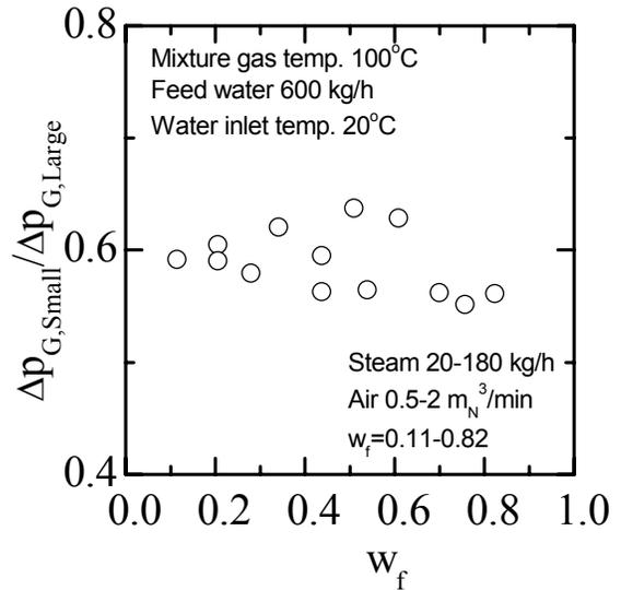
Fig. 7 Ratio of pressure loss in gas side at different steam concentration
