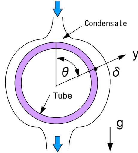
Fig. 1 Heat resistance of condensate film
