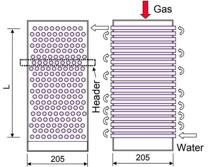
Fig. 3 Schematic of tube bank
