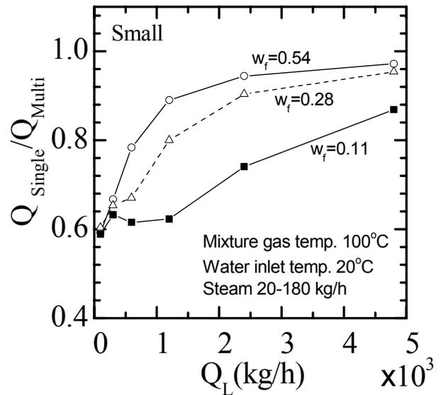
Fig. 11 Ratio of heat recovery at different water flow rate in “Small” HX
