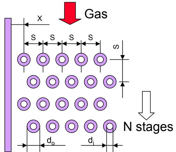
Fig. 4 Schematic of tube array
