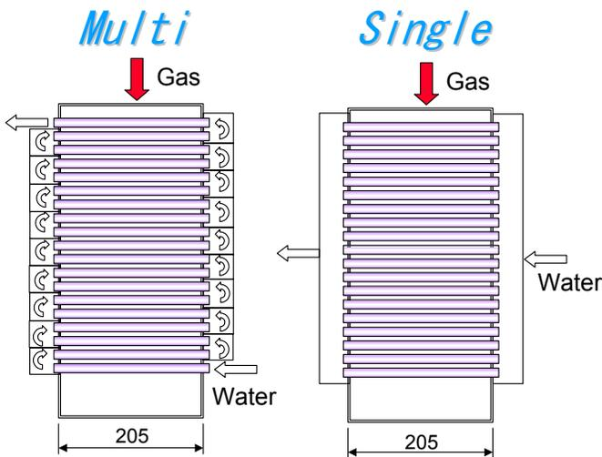
Fig. 9 Comparison of multi and single header
