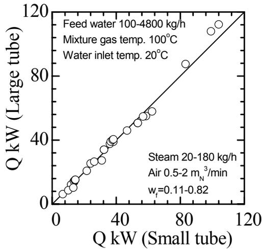
Fig. 6 Comparison of calculated heat recovery for “Large” and “Small” heat exchangers
