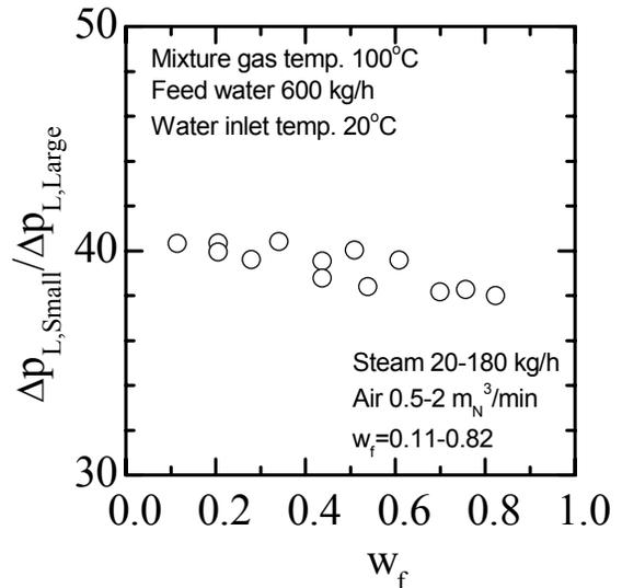
Fig. 8 Ratio of pressure loss in water side at different steam concentration
