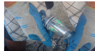
Lights attached to the nets create enough of a warning to alert sea turtles to a barrier
