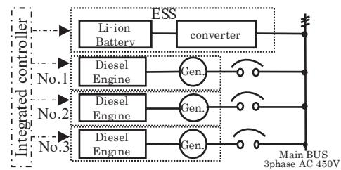
Fig.1 Onboard power system with ESS
