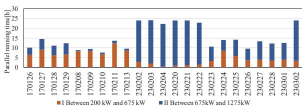
Fig.4 Parallel operation time of generators by electricity demand zone
