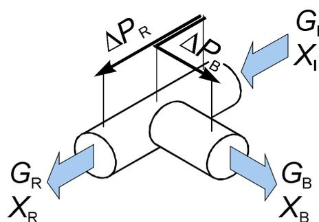
Fig. 3 Definition of variables for dividing two-phase flow at a T-junction
