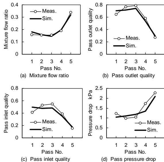
Fig. 5 Examples of simulation result (Condition: Flat heating,  $Q=450$  W,  $X_H=0.3$ )
