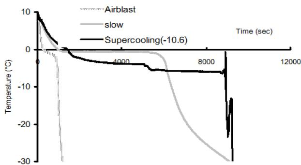
Fig.1.1 Freezing curves from the different freezing methods
