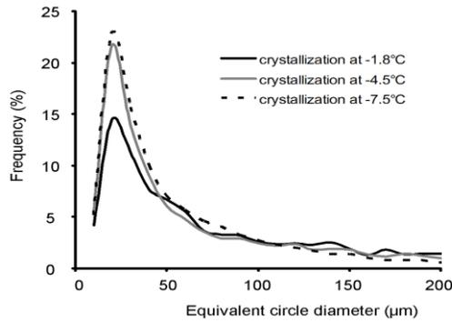
Fig.4 The distribution curve of the equivalent circle diameter of ice crystals that were frozen with the supercooled freezing method
