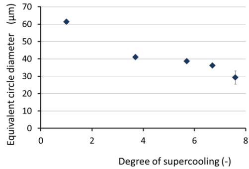
Fig.5 The equivalent circle diameter of ice crystals that were frozen with the supercooled freezing method at different degrees of supercooling
