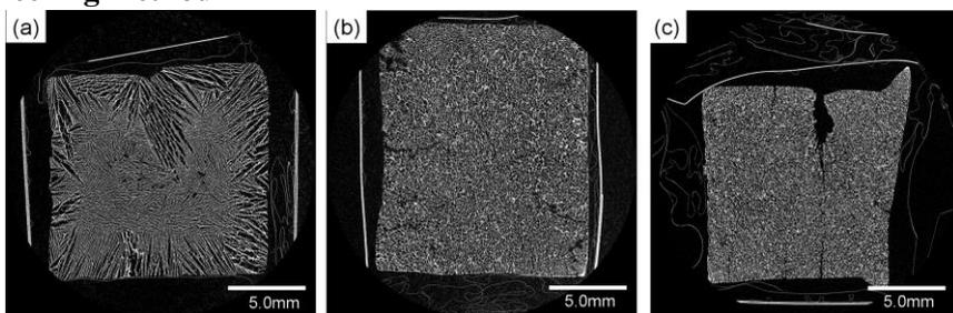
Fig.3 Cross-sectional images of the soy bean curds frozen by the supercooled freezing method. Ice crystallized at (a)  $-1.8^{\circ}\text{C}$ , (b)  $-4.5^{\circ}\text{C}$ , and (c)  $-7.5^{\circ}\text{C}$
