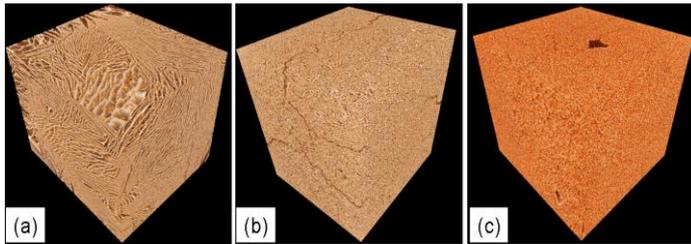
Fig.6 The 3D images of the soy bean curds frozen by the supercooled freezing method. Ice crystallized at (a)  $-1.8^\circ\text{C}$ , (b)  $-4.5^\circ\text{C}$ , and (c)  $-7.5^\circ\text{C}$
