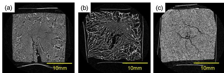
Fig.2 Cross-sectional images of the soy bean curds that were frozen by (a) the rapid freezing method, (b) the slow freezing method, and the (c) supercooled freezing method
