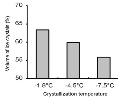
Fig.7 Volume of ice crystals frozen by the supercooled freezing method at different crystallization temperatures
