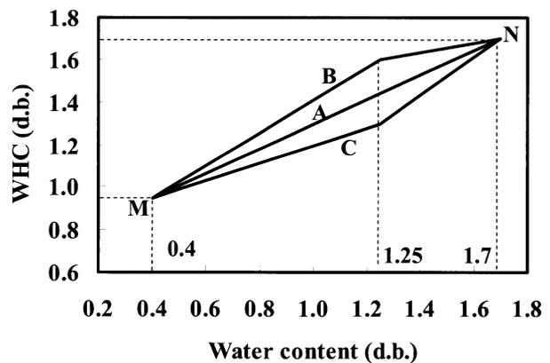
Fig. 2 WHC profile used for the calculation of transient water content profile in a slab of wheat flour dough during boiling. A: Linearly varying WHC profile, B: WHC profile with a breaking point at  $m = 1.25$  (d.b.), WHC=1.6, C: WHC profile with a breaking point at  $m = 1.25$  (d.b.), WHC=1.3. d.b. means dry basis (kg-water/kg-solid).
