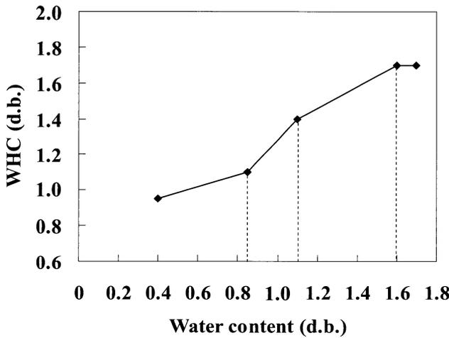
Fig. 5 WHC profile with three bending points (at  $m=0.85, 1.1,$  and  $1.6$  kg-water/kg-solid). d.b. means dry basis (kg-water/kg-solid).
