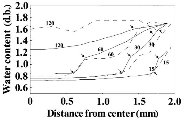
Fig. 6 Water content profile in a slab of wheat flour dough calculated using the WHC profile given in Fig. 5, is compared with the measured profile. The numbers indicate boiling time (min). d.b. means dry basis (kg-water/kg-solid). ——— calculated profile, - - - - - measured profile. Arrows indicate bending points in transient water content profiles.
