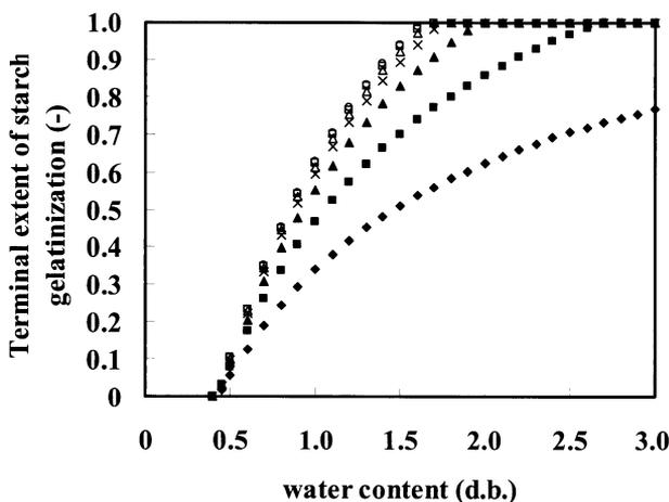
Fig. 1 Terminal extent of starch gelatinization values plotted against water content (calculated from the published data of Fukuoka *et al.* [11]). ◆70°C, ■75°C, ▲80°C, ×85°C, △90°C, □95°C, ○100°C. d.b. means dry basis (kg-water/kg-solid).
