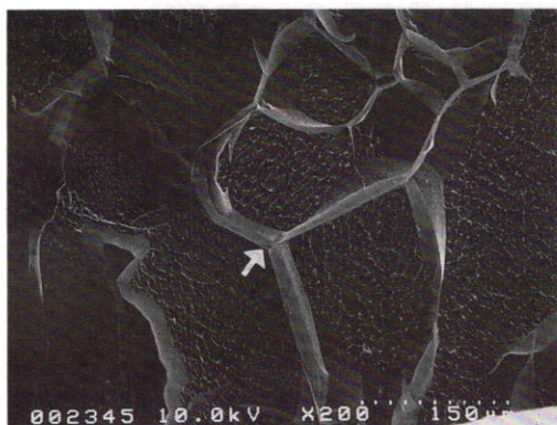
Fig. 2. A Cryo-SEM photograph of the internal surface of a 1% agarose gel at -80^\circ\text{C} , at 200 magnifications. The sample has never been thawed. The white arrow indicates the deltoid void among the compartments; \circ , the trace of sublimed ice crystal.
